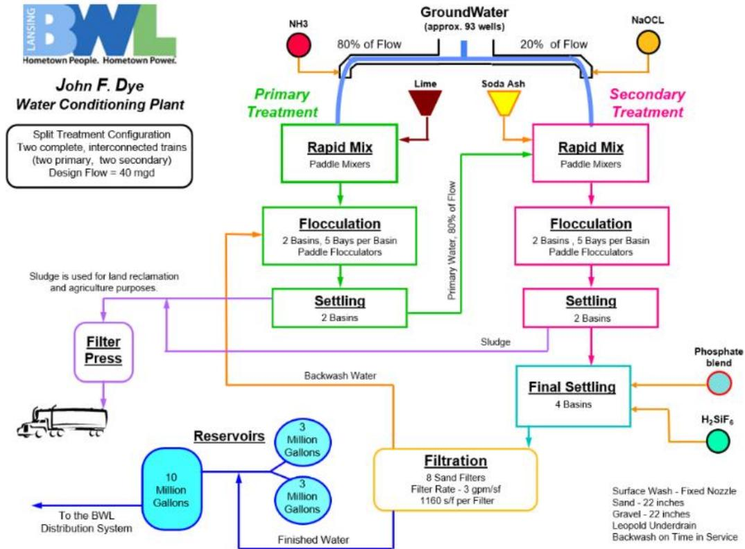
Figure 9 - Dye WCP Treatment Process
