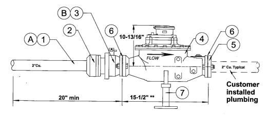
\*\* Allows room for two 1/8" thick gaskets
